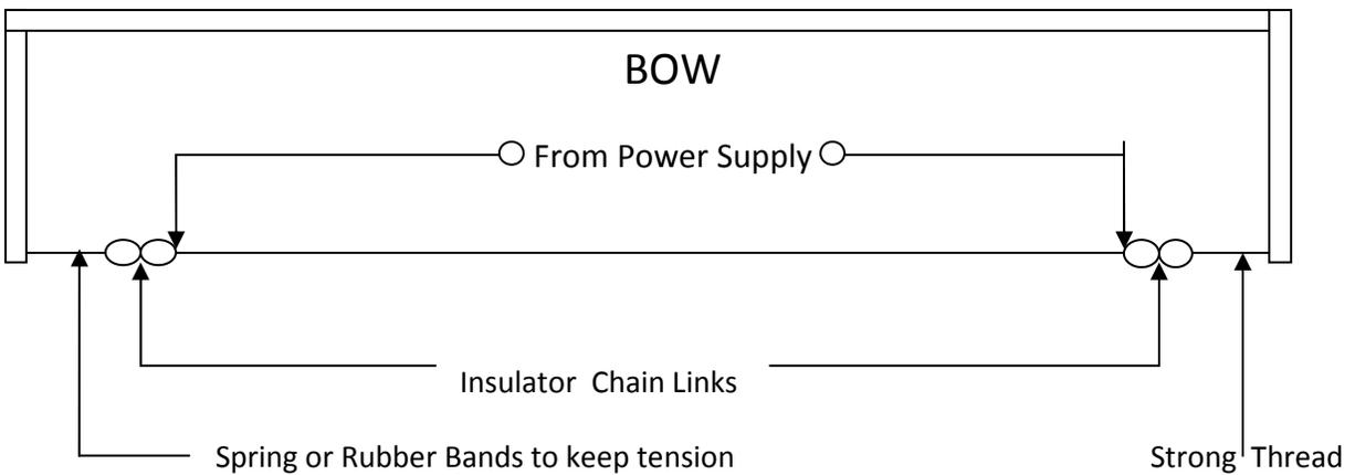
Crocodile Clips can be used to connect Power Supply output to the cutting wire ends on the bow.
