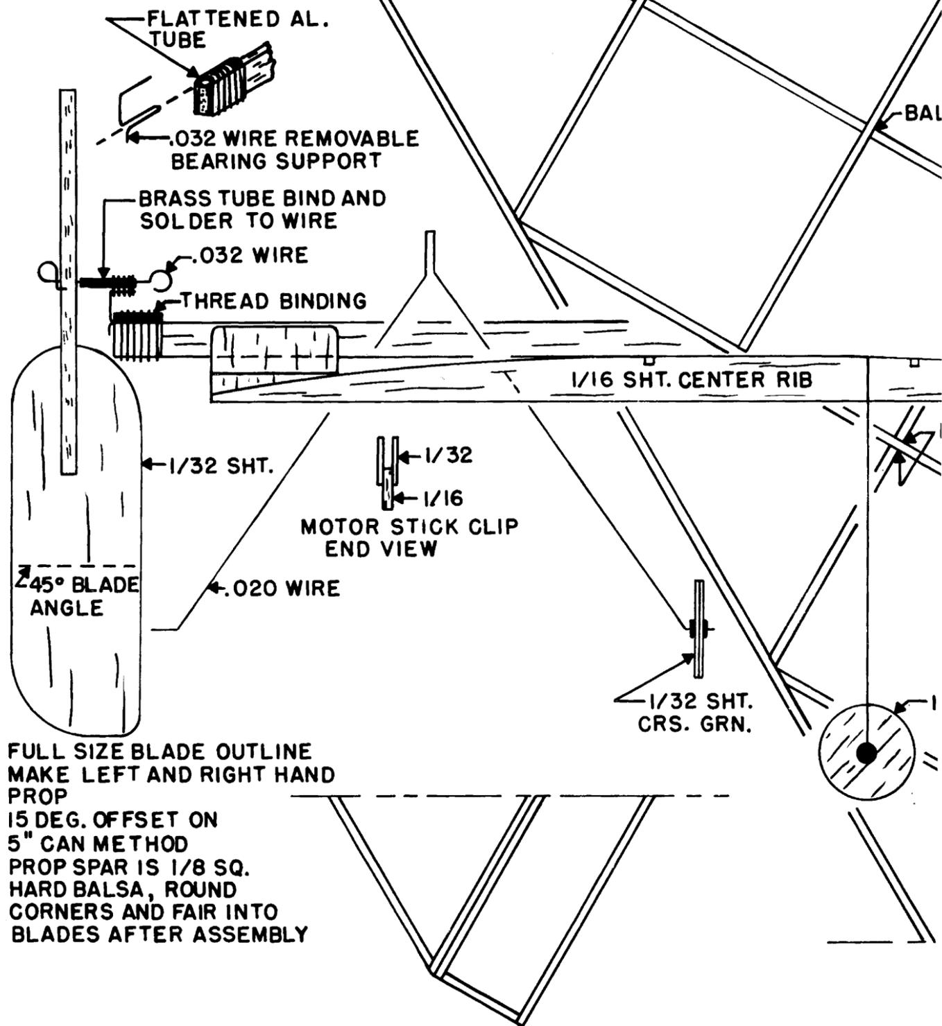
LEAD AND WING, TRAILING EDGES PARTS ARE 1/16 SQ.
